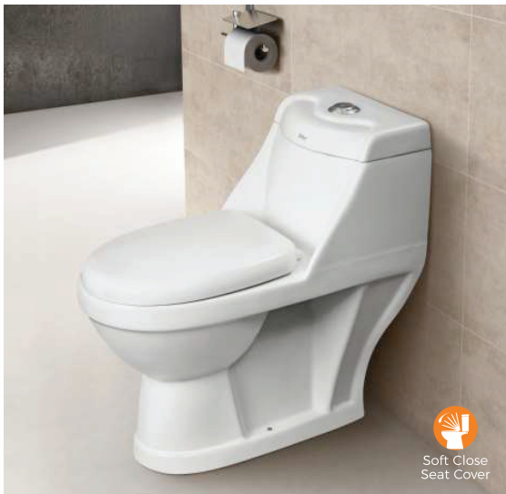
renesse Code 1049 L 720 W 375 H 660mm / L 28.5" W 15" H 26" Wash Down S-trap Central of outlet to wall 220mm (9")
